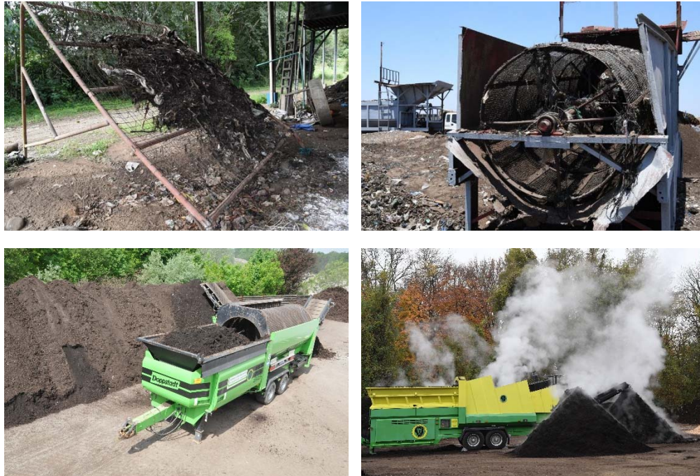
Fig. 11. Example of an artisanal sieving system of two drum sieve and a star sieve.
