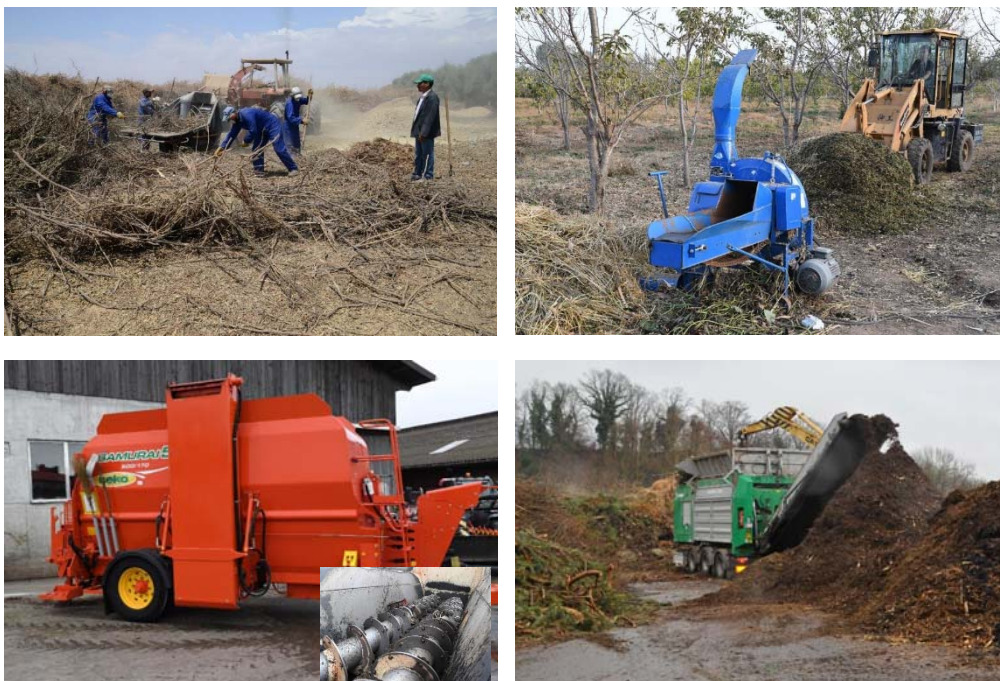
Fig. 9. Example of shredders for the compost plant.
